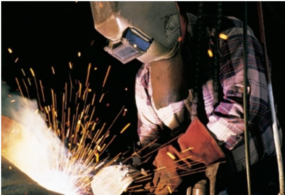
Figure 4.27 Welders use a dark mask to protect their eyes and to see white-hot joints clearly.
